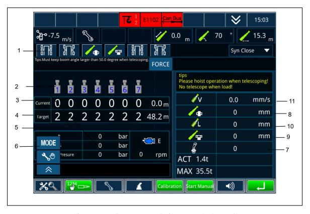
Figure 4-36 Boom status during manual telescoping
