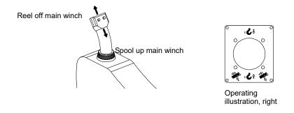
Figure 4-57 Spooling up / reeling off main winch
