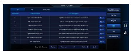
Figure 3-14 ABS fault view
