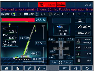
Figure 4-45 Remaining unlocking time display, main interface
