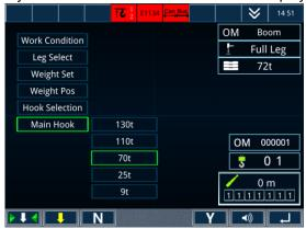
Figure 4-25 Main operating mode setting interface
