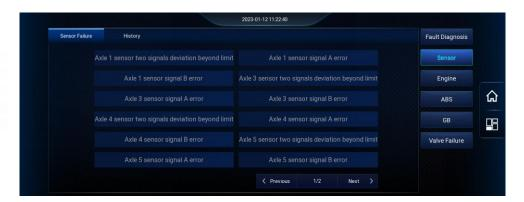
Figure 3-12 Sensor fault view
