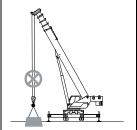
j) When the load is off the ground, the operator must stay in the cab.
