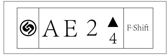
Figure 3-45 FAST transmission gear position display
