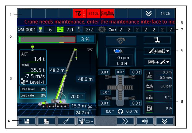
Figure 4-10 Crane working status monitoring interface
