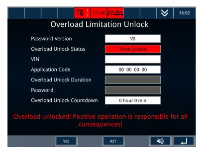
Figure 4-43 Serious overload time-limited unlocking interface
