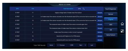
Figure 3-11 Engine fault view
