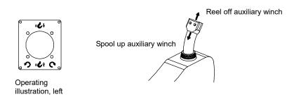
Figure 4-58 Spooling up / reeling off auxiliary winch
