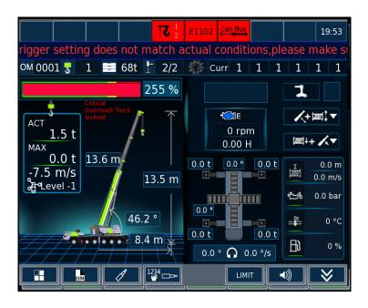
Figure 4-42 Main interface serious overload warning prompt
