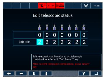
Figure 4-34 Current boom status modification
