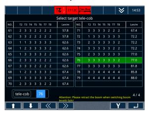
Figure 4-27 Telescoping combination selection interface
