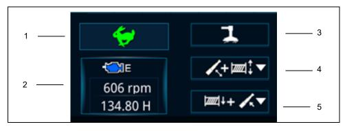
Figure 4-21 Speed and function buttons
